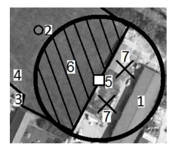
**Figure 2.** Section of chosen farm (1 - barn for housing cattle; 2 - location of centralized drinking troughs; 3 - pasture fencing; 4 - pasture; 5 - IQRF unit; 6 - monitored area; 7 - unmonitored area).
