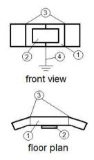
**Figure 3.** Scheme of shielding pad (1 – shielded pad; 2 – space for placement of the IQRF unit; 3 – shielding flaps with adjustable angle; 4 – electrical grounding).
