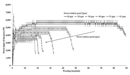
Figure 2. Effect of screw rotation speed on electric power input of duo press and pressing time for 10 kg of rapeseeds.
