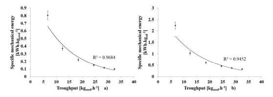
Figure 3. Dependence between seed material troughput and mechanical energy for a) pressing one kilogram of rapeseeds; b) obtaining one kilogram of oil.
