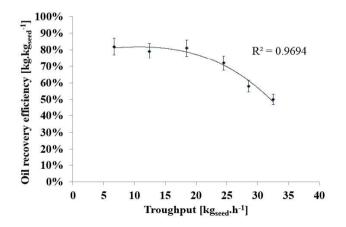
Figure 4. The effect of seed material troughput on oil obtained ratio.
