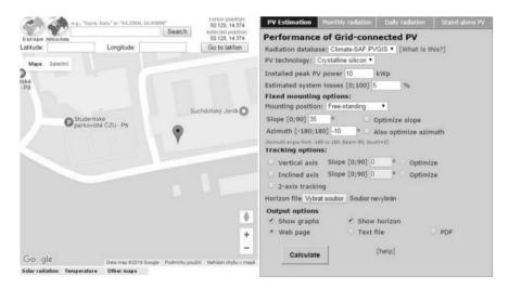
Figure 2. GUI of PVGIS with parameters for PV installation in Prague.
