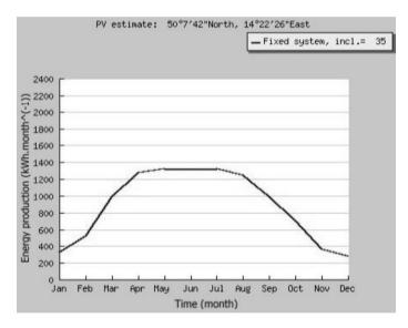
Figure 3. PV estimate for installation in Prague on the CULS campus.
