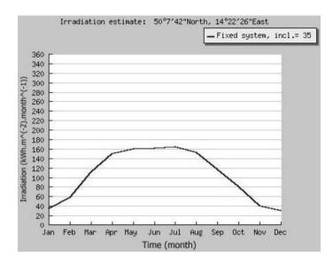
Figure 4. Irradiation estimate for Prague.
