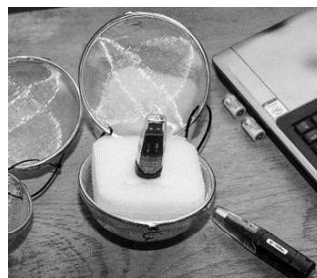
Figure 2. Placing a datalogger into a protective sieve.
