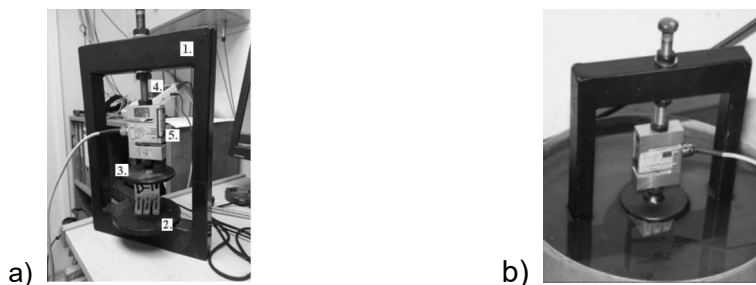
Figure 4. Swelling pressure measurement equipment with CWM sample in height direction (marked as D): a – sample before immersion in water; b – sample in a time of testing; 1 – frame; 2 – lower support; 3 – upper support; 4 –screw; 5 – load cell.
