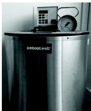
Figure 3. An apparatus for measuring vapour pressure.
