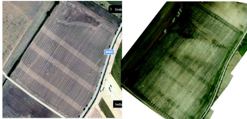
Figure 1. Satellite image (left) showing 1 pass (compacted) area for RTF simulation and orthophotograph (right) during vegetation with visible difference in compacted and non-compacted area.
