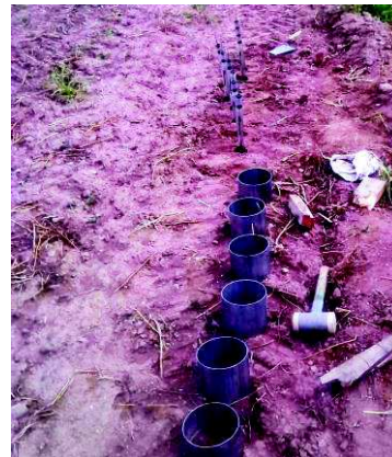
Figure 1. Measurements by Mini Disk infiltrometer and by Single Ring.
