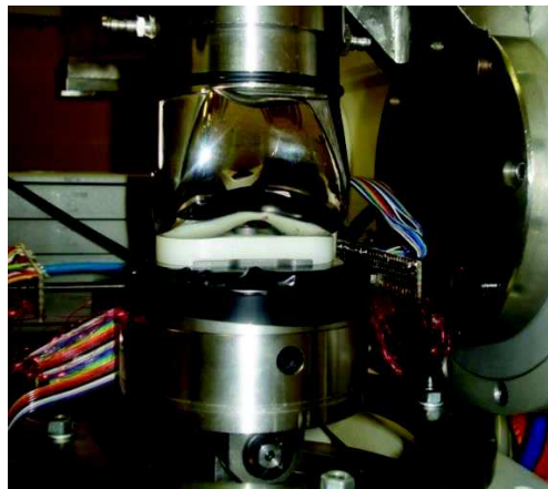
Figure 2. Knee movement simulator machine.
