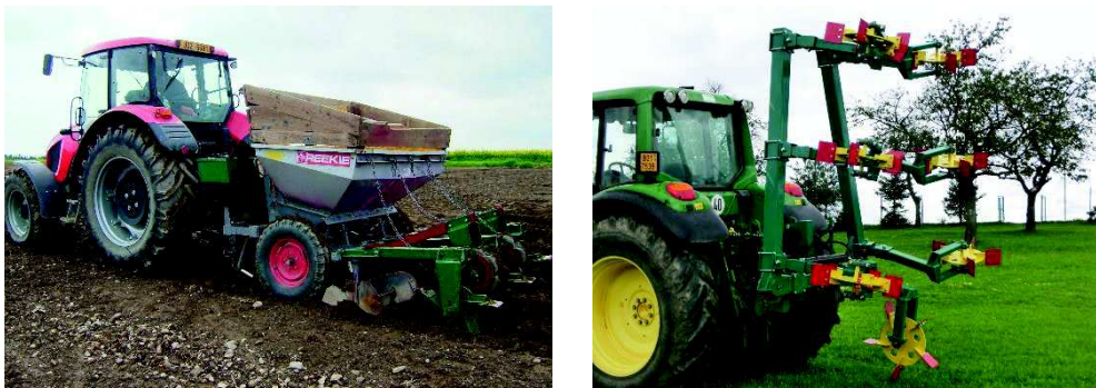
Figure 1. Reekie 2-rows planter with tied ridging adapter and KOVO NOVAK 6-rows tied ridger.
