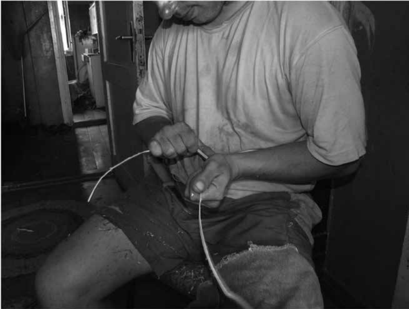
Figure 3. Prit Retsep demonstrating how to make splits by riving a stick. For the first 10 cm, he uses his knife; after that he drives the rift with his hands, using his fingers and palm to direct it – the rift will run to the side that the stick is bent to. Photograph by Madis Rennu (2010).
