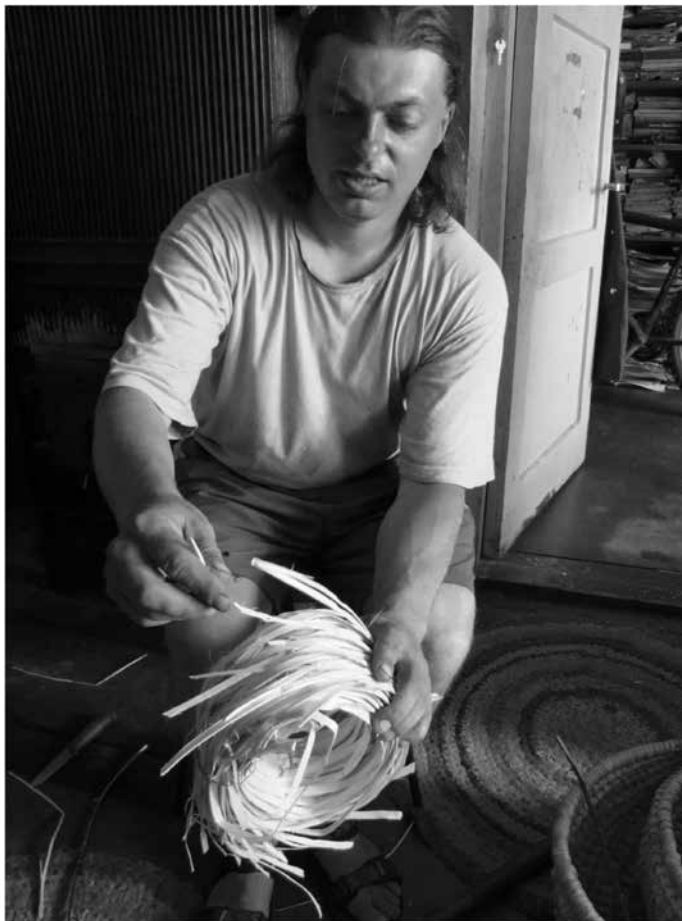
Figure 4. A roll of splits riven from a stick even thinner than the one shown in Figure 1. Before weaving, the roll must be left to soak in water for an hour. Photograph by Madis Rennu (2010).
