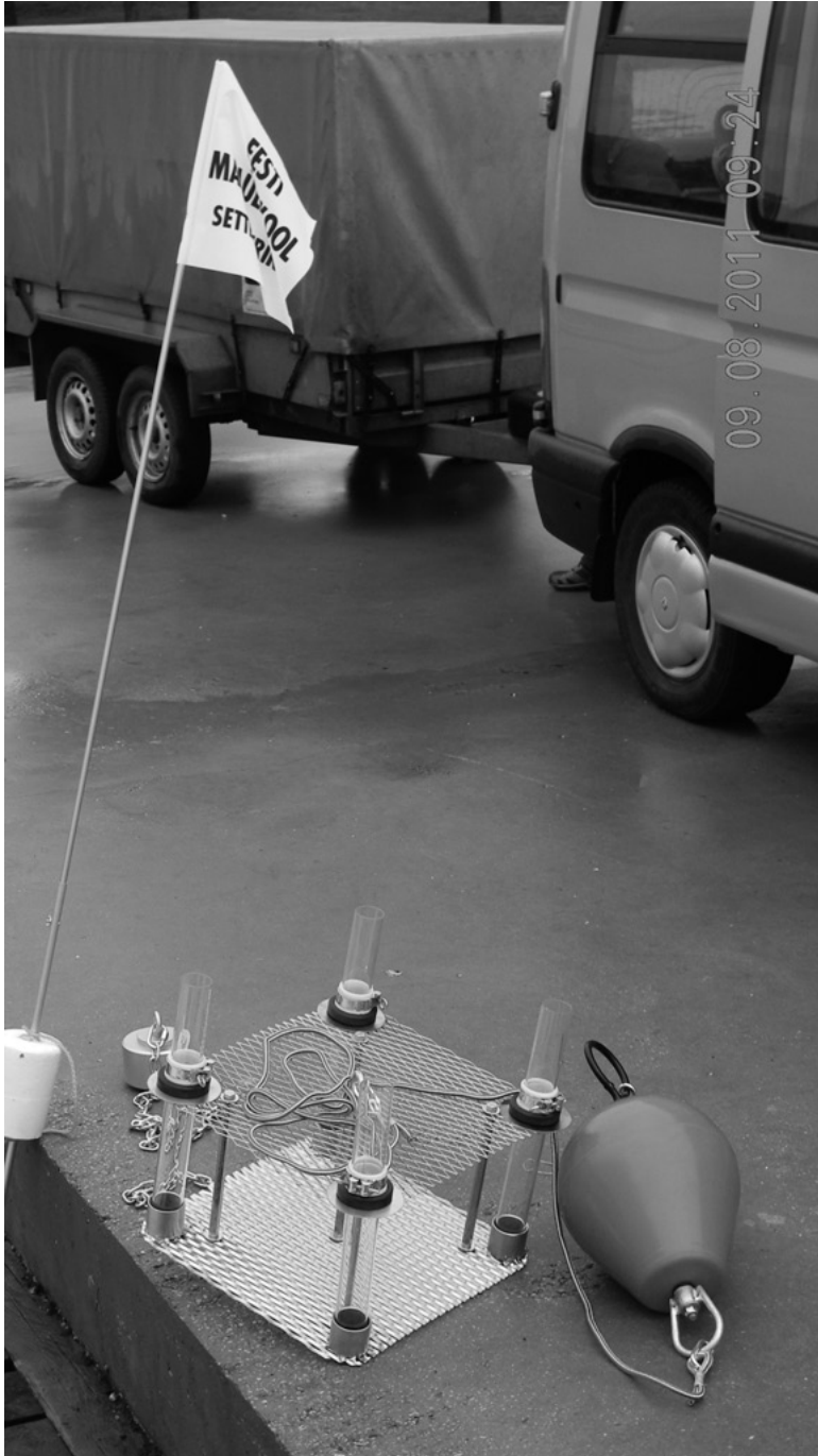
Figure 2. Sediment traps were used in the Enonselkä basin of Lake Vesijärvi and in Lake Peipsi to quantify the rates of gross sedimentation and sediment resuspension (photo by Aivar Roomet).
