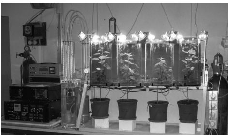
Fig. 1 Photograph of the computer-controlled growth chamber and gas exchange system used to control the ambient [\text{CO}_2] during canopy development.
