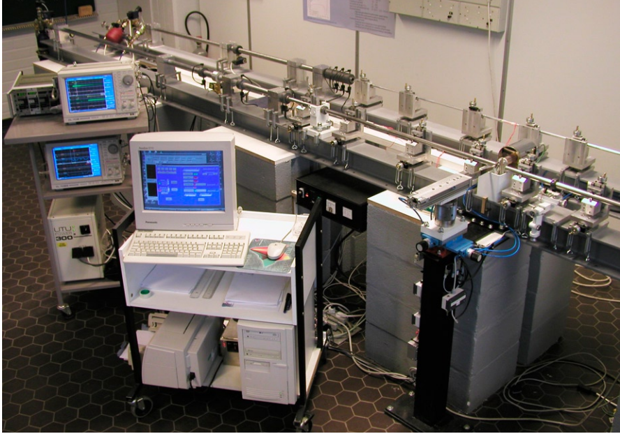
Figure 6. The compressive SHPB equipment at TUT. The computer together with components of the data acquisition system (DAQ) is seen at the front. The set up of pressure bars together with stanchions built on the I-beam are just behind.
