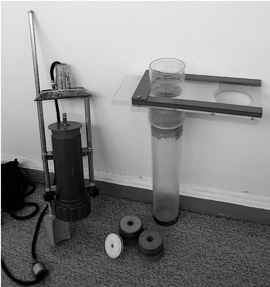
Figure 4. A Willner-type gravity corer was used for sample collection in PAPER I , photo by A. Kisand.
