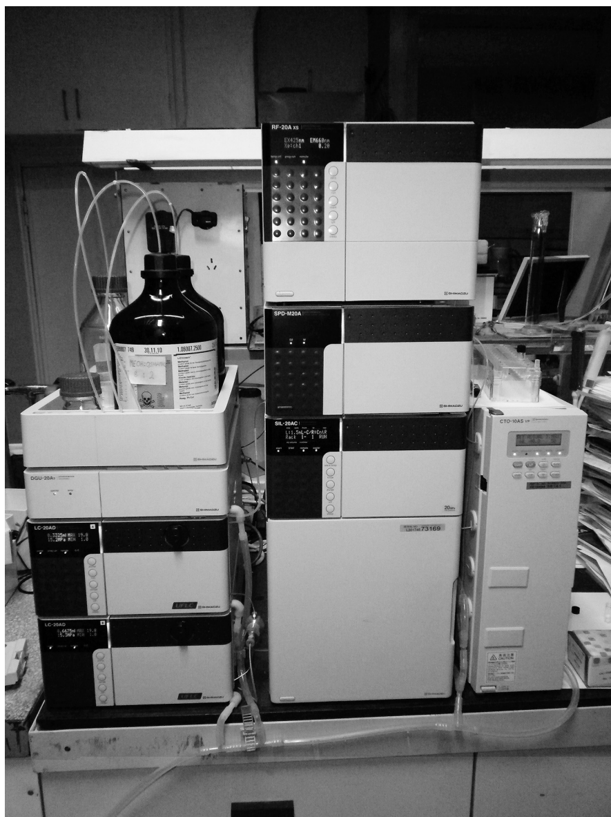
Figure 5. Shimadzu Prominence series HPLC system with degasser, two high pressure pumps, autosampler, column oven and photodiode-array (PDA) and fluorescence detectors that was used in phytoplankton pigment analysis in PAPER I .
