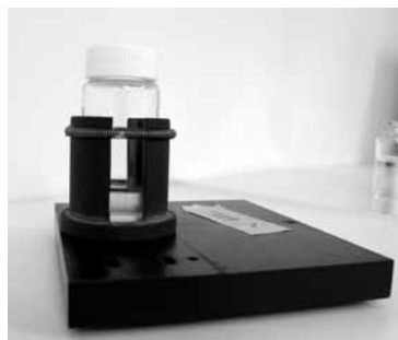
Figure 5. Vial (20 ml) holder for direct optical density measurement from the culture vessel
