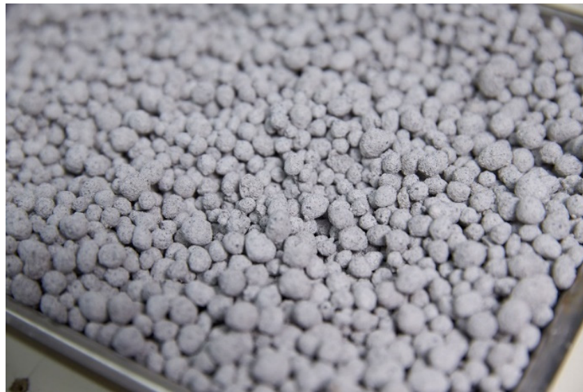
Figure 11. Pilot samples of artificial fine aggregates produced using B/S0.4 after 28 days of curing.
