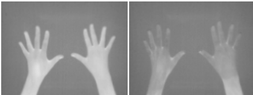
Fig. 2: Exemplary greyscale representation of thermal images taken before (left) and after (right) disinfection with dorsal side facing up
