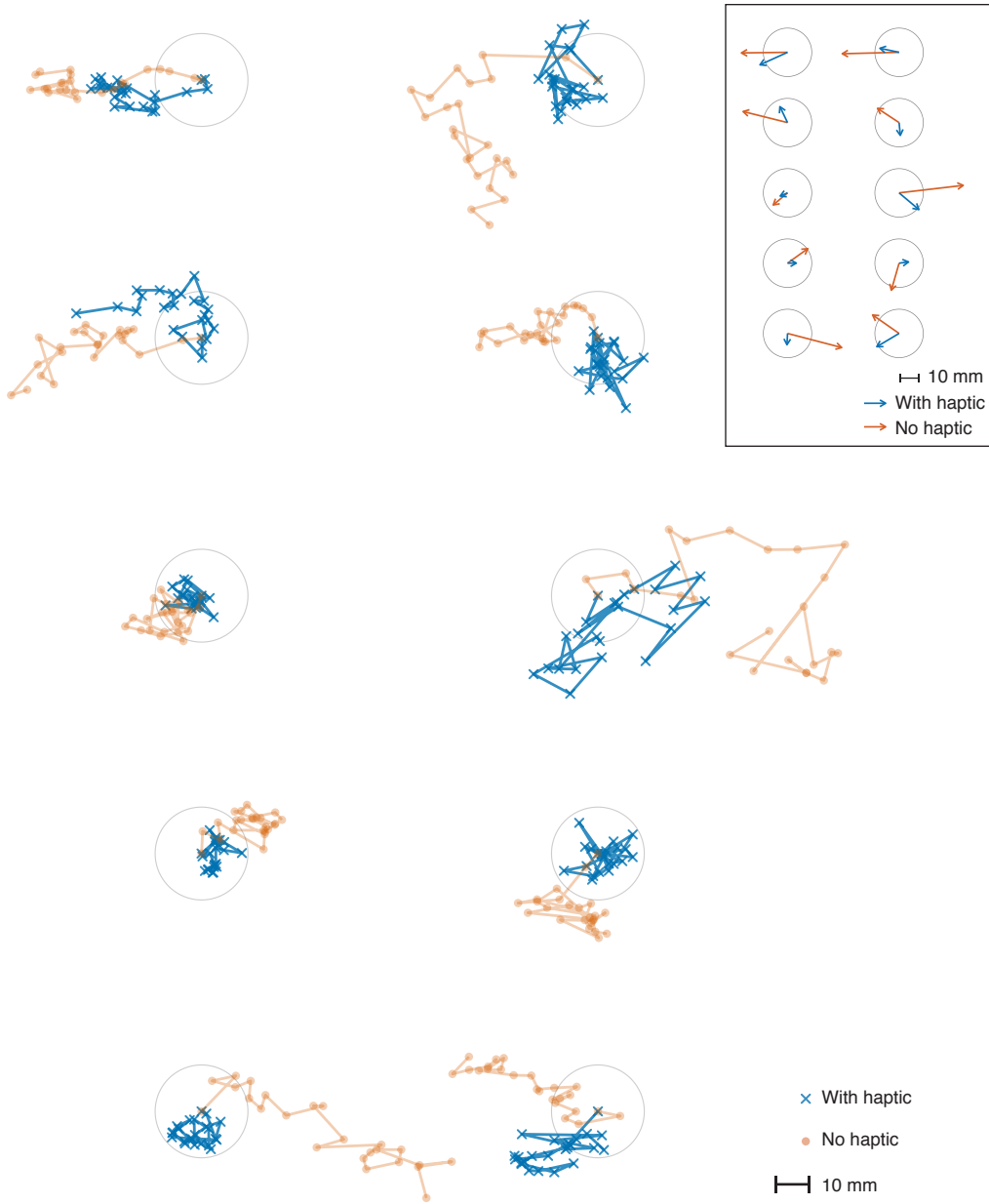
Figure 5.5: Contact points from each of the ten participants. The haptic feedback apparently reduces drifts. Only left targets were shown. Subsequent trials are connected with a line. The circle represents the button that is visible to the participants. The first trial always started at the center of the button. The inset shows the average direction and distance of these contact points.
