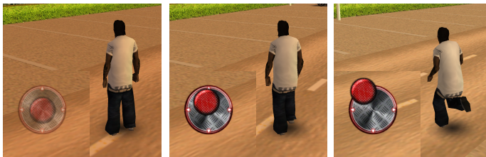
Figure 1.2: Touch screen virtual analog joystick can be controlled without lifting the thumb from the screen, hence, suffer less from space inaccuracy. (Image from Urban Crimes, Gameloft)
