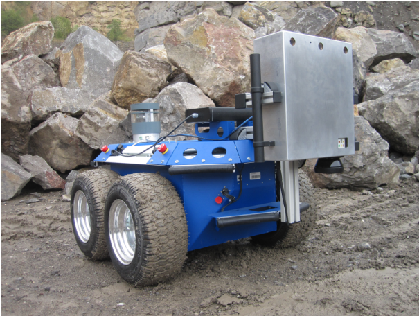
Figure 8. Self-contained localization unit mounted on mobile robot.
