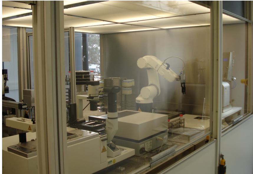
Figure 1.1.: A picture of the StemCellFactory ( www.stemcellfactory.de ) which was developed and build up within the StemCellFactory project. The six meters long and more than two meters wide machine was constructed at RWTH Aachen and is now located and maintained at Life & Brain GmbH in Bonn. It was designed for a fully automatic reprogramming of fibroblasts into iPSCs and a subsequent differentiation of these into neural cells and cardiomyocytes. One essential step in the StemCellFactory is the quality control of the end products in order to assure their usability as an in vitro disease model.
