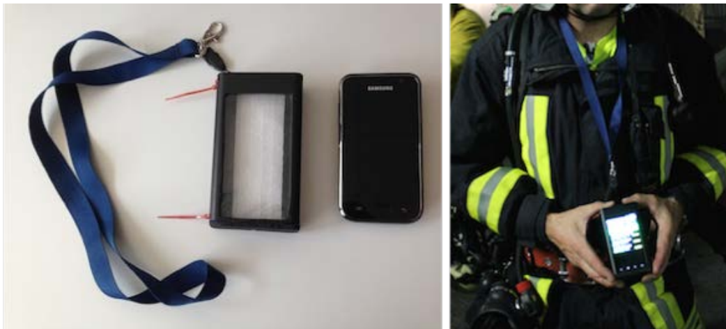
Figure 41 Boxed Seeker phone and wearable box to hang around the neck
