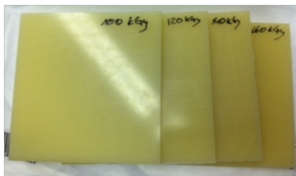
FIGURE 3.5: PE samples treated with \beta -radiation.
