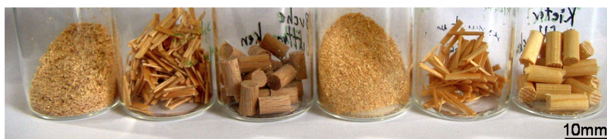
Figure 3.1. The individual fractions of wood utilized in the experiments; beech left, spruce right, the pine blocks are the sample on the right. The particle sizes are 0.1 - 0.5 mm, 10 \times 2 \times 1 mm 3 and 5 \times 10 mm 2 (picture made by Schlüter, 2011).
