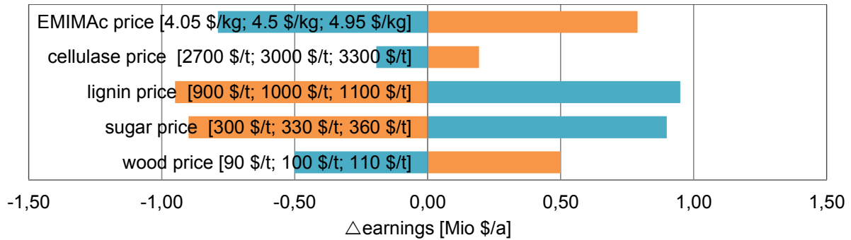
Figure 5.7. The result of a sensitivity analysis of raw material prices varying one parameter by 10% one at a time. Blue bars result from positive deviations in the raw material price, while negative ones are shown in orange.
