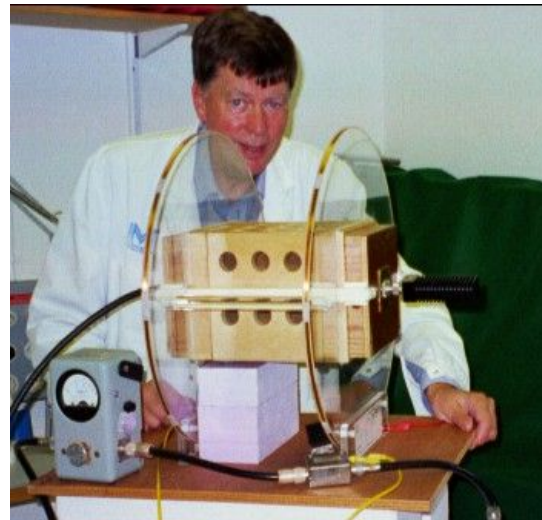
Figur 2 Our exposure system for Fischer rats.
