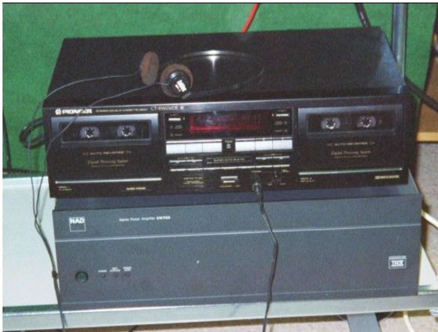
Figure 3 Cassette recorder with output signal connected to a sound power amplifier. The Helmholtz coils are connected to the amplifier's speaker output. The signal cassettes were obtained from Litovitz.
