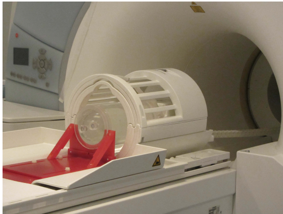
(a) Picture of a cylinder phantom transaxially centered within the MR head coil.
