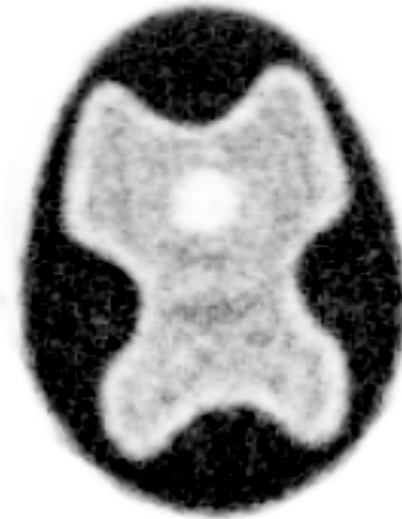
(b) Two chamber phantom reconstructed with 200 ML-EM iterations.
