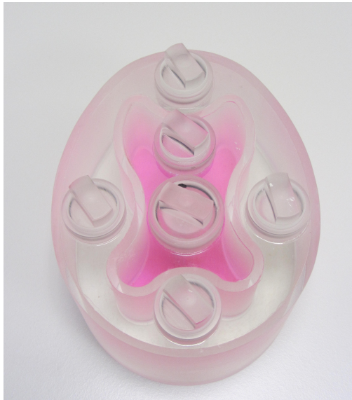
(a) Picture of the two chamber phantom.
