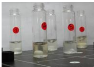
Figure 34. Reaction vessels standing on a magnetic stirring board and filled with the reaction mixture for hydroxylation of selected benzene substrates. The photo was taken after 2 h reaction prior to extraction of products for GC-FID and GC-MS analysis.
