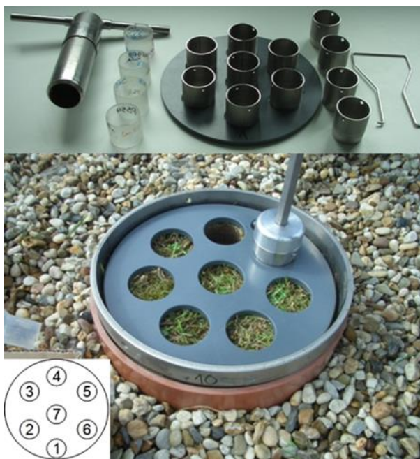
Figure II-10: Sampling equipment for TME (pre-study and range-finding study) (right side) and in the field (left side). Tools were made by the University's own facilities. Calibration disc used for the TME pre-study, the range-finding study and the dose-response study. The modified soil corer with plastic inlays was used from the dose-response onwards.
