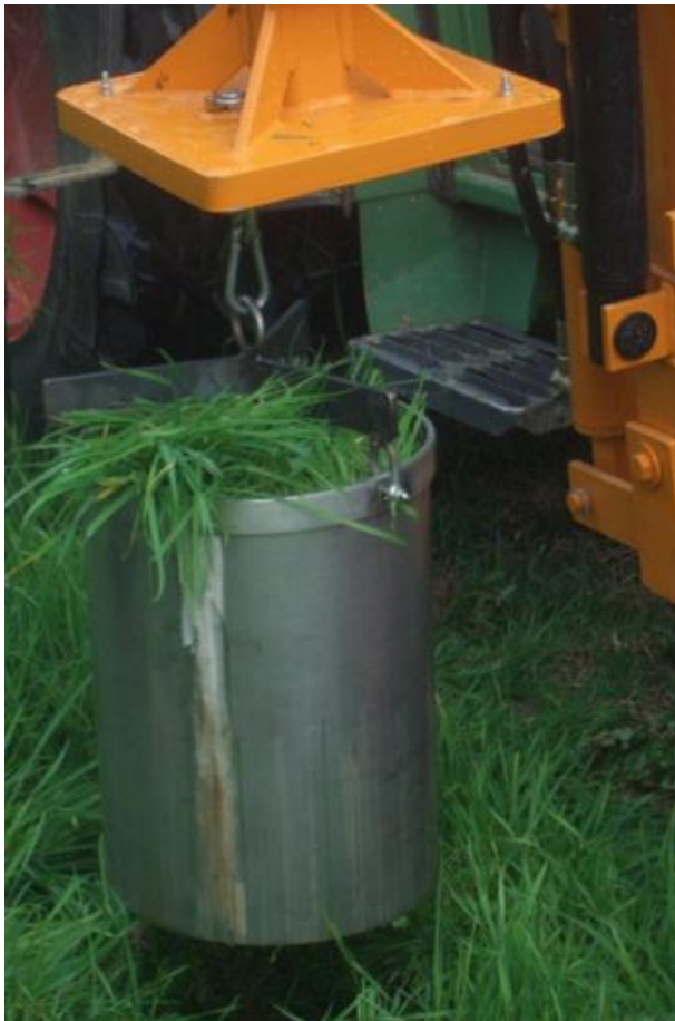
Figure II-3: Soil coring by means of a hydraulic pile pusher.
