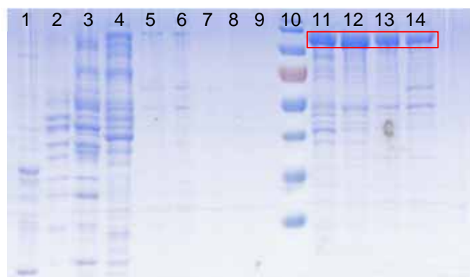
Fig. 92: SDS-page of the collected fraction during purification. Lane 1-4: fraction before protein elution; Lane 5-9: fraction after protein elution; Lane 11-14: protein elution fraction, red frame indicates P450 BM3 at 120 kDa; Lane 10: prestained protein ladder.
