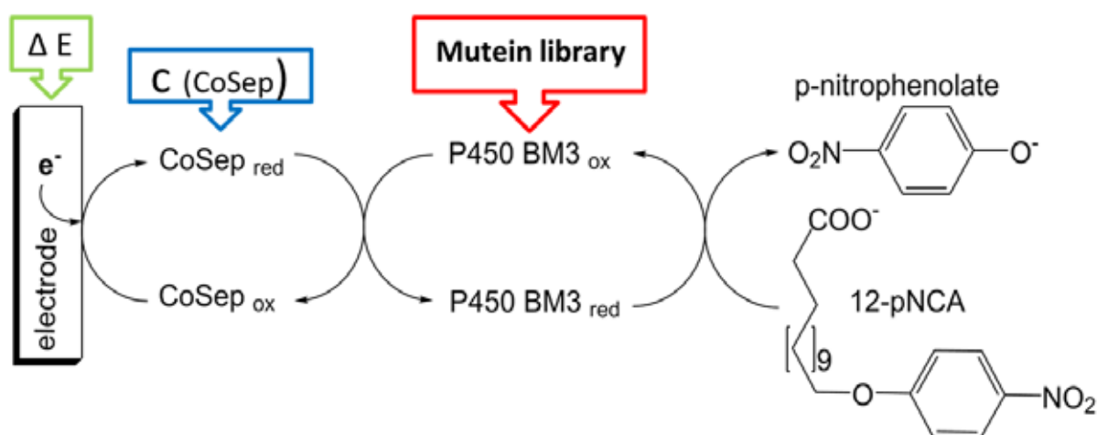
Fig. 4b: Reaction scheme of the electrochemical driven conversion of pNCA by P450 BM3 with CoSep as mediator.
