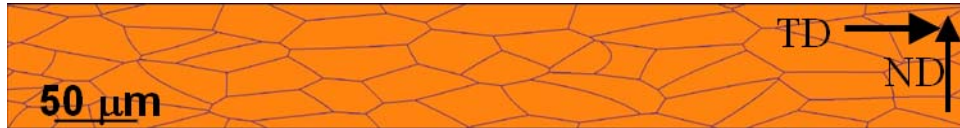
Fig. 78 The calculation domain for phase field simulation on the cross section of a rolled strip.
