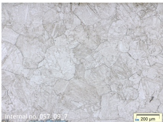
Fig. 27 The austenite grains in the Mn-Mo DP steel revealed by the quenching and etching method after the austenitisation at 1200 °C and 1150 °C
