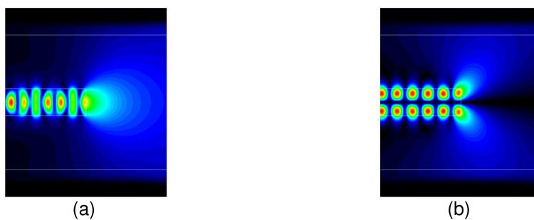
Fig. 6. Propagation field distribution obtained by FEM analysis with POM boundary conditions corresponding to the problem shown in Fig. 5: (a) fundamental and (b) first higher order TE modes.
