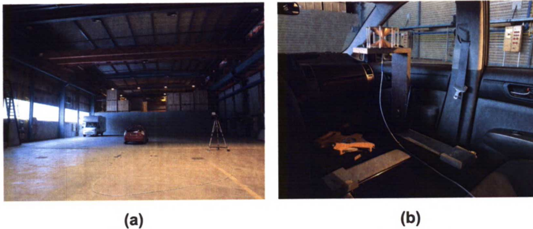
Figure 4.9 Inside-outside measurements depicting (a) RX around car (b) TX on 2D scanner inside car
