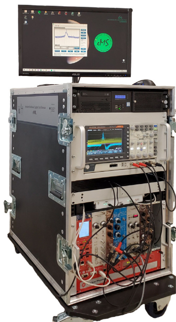
Fig. 3. A photo of the current electronic rack. The flight case includes a NIM crate with data acquisition modules (SCA, MCA, velocity unit), computer, oscilloscope, HV unit.
