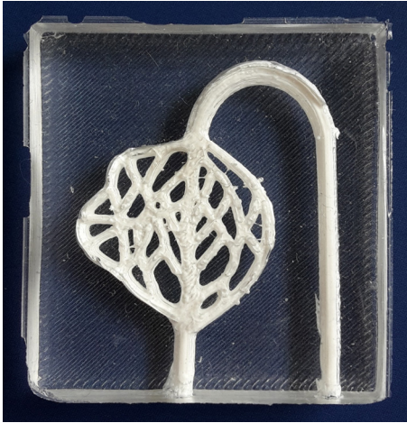
Figure 2: Photograph of the 3D printed vessel phantom; edge length = 45 mm.
