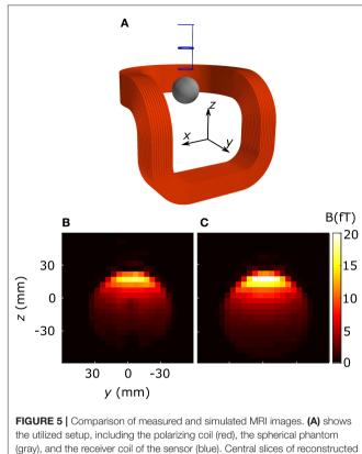
(gray), and the receiver coil of the sensor (blue). Central slices of reconstructed images, not corrected for the sensitivity profile, are presented for measurement **(B)** and simulation **(C)**. Please note that the actual phantom contains a mount for dipolar current electrodes, which is recognizable in the central lower half of the reconstructed measurement, but was not accounted for in the simulations.
