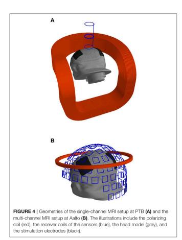
gradient-echo sequences can be simulated for arbitrary imaging objects. Both the polarizing field profile and the coupling of the magnetization to the sensor (Equation 2) were calculated by analytically integrating the Biot–Savart formula over line segments [20, 25].
