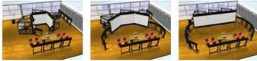
Figure 9: Three position adjustments possibilities of CAVE screens (90°/135°/180°).
