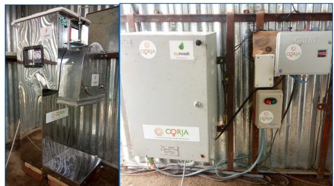
Oorja introduced a new agroprocessing service and operates two mills integrated with solar pumps. Photo shows the processing mill (left) and associated electronics (right) required to integrate the mill with the solar pump. Photo courtesy of Oorja.
