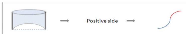
Figure 12. Schematic view of the silicone membrane ring and respective pressure deflection curve.
