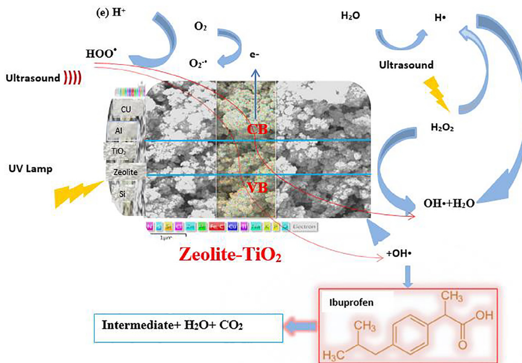
Fig. 10. The proposed mechanism for ibuprofen removal by the “Zeolite-titanium-H 2 O 2 -UV-ultrasonic” system.
