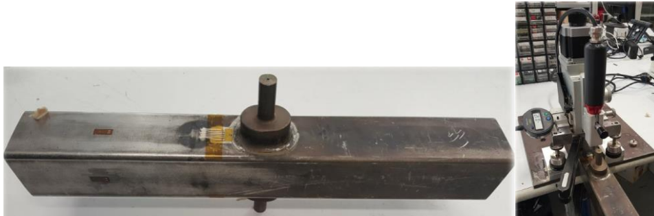
Figure 3. Left: workpiece (sample “2P”) equipped with the CCW - type B strain gage rosette; right: test configuration for the measurement of residual stresses based on ASTM E837
