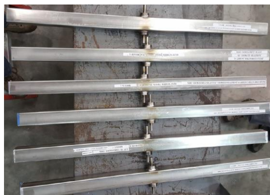
Figure 2. Prototype CS Helium Inlet specimens in the as-received condition for further processing and testing by NHMFL [5]
