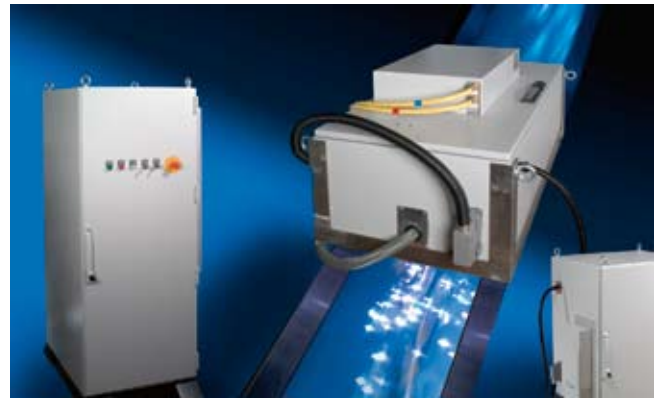
5 Laser unit for single particle analysis on belt conveyors; left: Control cabinet, centre/top: Laser module, centre/bottom: Belt conveyor with sorting material and laser-induced plasmas (long-term exposition), right: Spectrometer module
