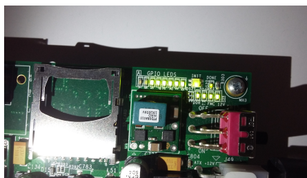
Figure 19: Status LED after Xilinx board initialization.
