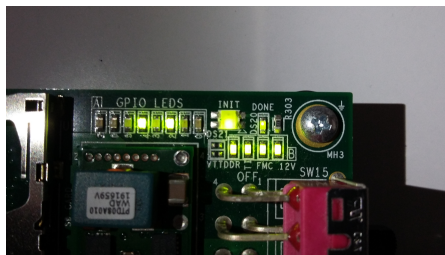
Figure 17: Status LED after Xilinx board initialization.
