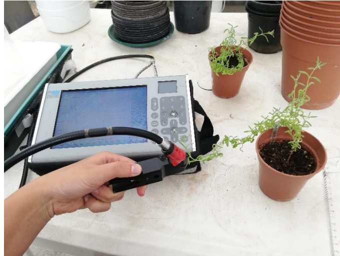
Figure 3.2 – Lavandula stoechas reflectance measurement using a spectroradiometer.
