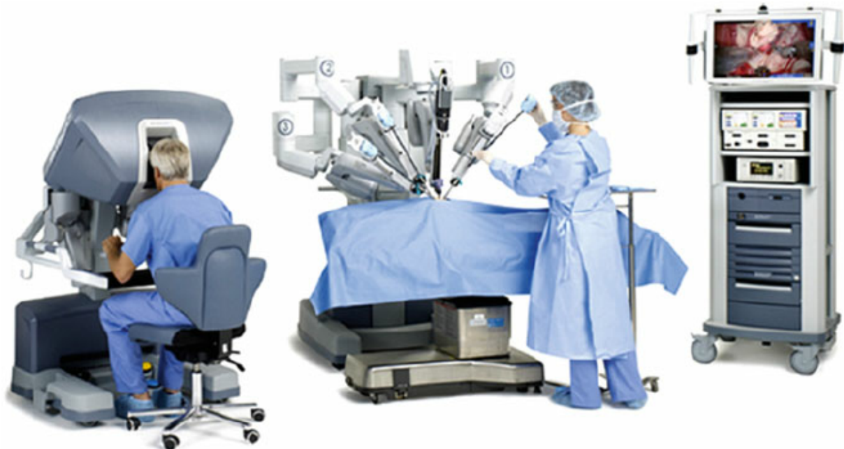
Figure 4.1: Representative image of the different elements that make up the da Vinci surgical system. On the left, the console where the surgeon controls the movements of the robotic arms; in the center, the various robotic arms responsible for performing the tasks given by the surgeon; on the right, an element that allows the entire team on the block to follow the surgery not only visually but also with audible guides.
