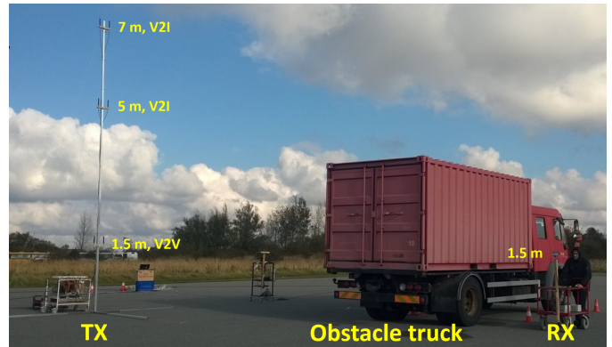
Fig. 1. Measurement scenario and setup with stationary TXs deployed at 1.5 m (V2V configuration), 5 and 7 m (V2I configuration), large vehicle obstacle (truck), and moving RX at 1.5 m.
