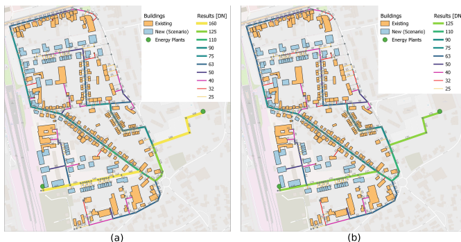
Figure 1. Results of the district heating network optimization with two energy supply plants. DN: nominal diameter. (a) Sizing of the piping system without decentral storages. (b) Sizing of the piping system with decentral heat storage of 1 m 3 at each customer. The decentral heat storages permit a smaller diameter at the distribution lines due to peak-shaving. Background map: OpenStreetMap contributors.
