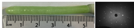
Figure 11. Boule of \text{Tm}_2\text{Si}_2\text{O}_7 prepared by the floating zone method in air atmosphere, at ambient pressure, in a flow of air of 1–2 L/min, using a growth speed of 10 mm/h. Also shown is the X-ray Laue pattern of one of the sides of the \text{Tm}_2\text{Si}_2\text{O}_7 crystal boule.
