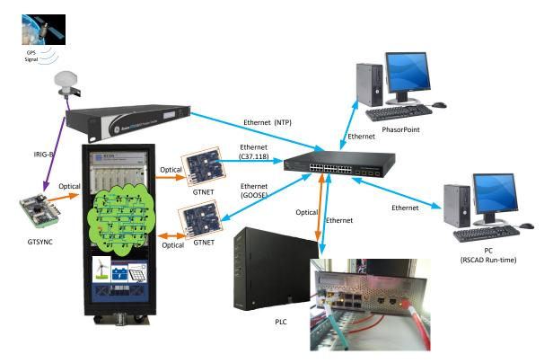
Figure 6-2: RTDS testbed architecture and communication infrastructure.
