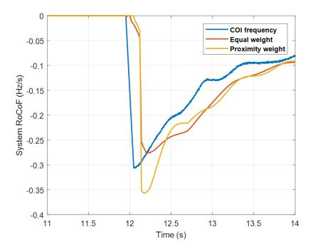
Figure 8-23: System RoCoF of different PMU weight configurations
