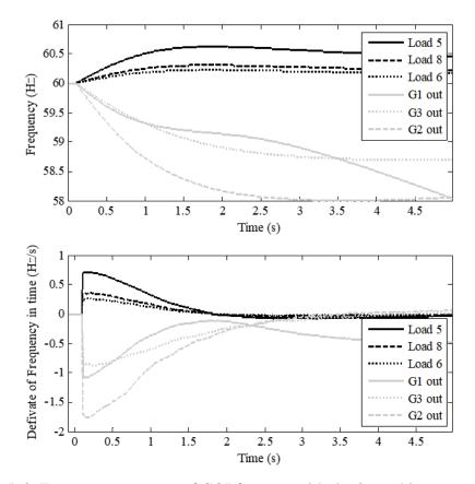
Figure 5-6: Frequency response of COI for tests with the 3-machine tests system.
