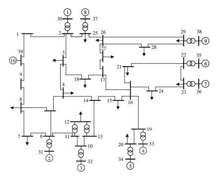
Figure 7-4: IEEE 39-bus test system.
