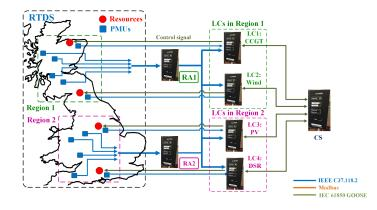
Figure 8-6: Test setup for validation of the EFCC scheme.
