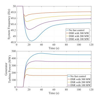
Figure 4-7: Simulation of a 500 MW generation loss in IEEE 39-bus test system with varying amounts of FFR.
