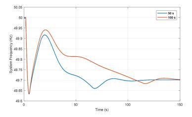
Figure 8-10: Simulation results of a 1000 MW load increase at bus 9 of region 1 with two different service pulling off speed.
