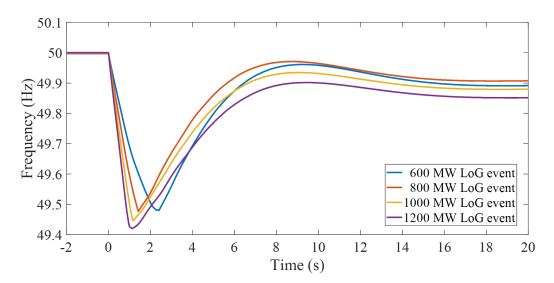
Figure 7-6: The frequency response of the proposed UFLS scheme following LoG events of different size.
