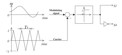
Figure 3-5: The pulse-width modulation (PWM) switching strategy.
