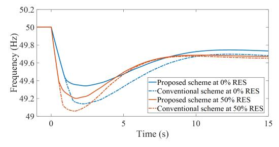
Figure 7-7: The frequency response of the proposed UFLS scheme following LoG events of different size.
