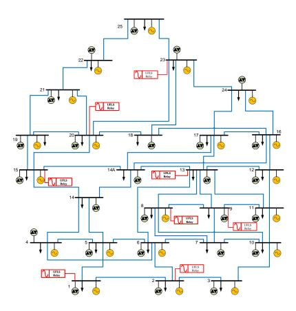
Figure 7-10: Single-line diagram of GB test system in RTDS.
