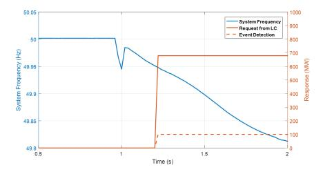
Figure 8-11: Simulation results of a 1000 MW load increase at bus 9 of region 1.
