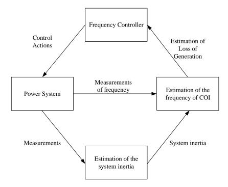
Figure 1-1: Depiction of the main stages of the adaptive frequency control.
