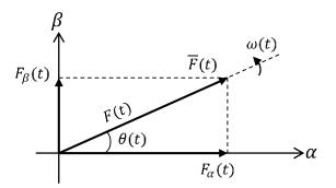
Figure 3-7: Space phasor in the stationary reference frame.
