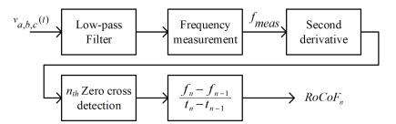
Figure 7-2: Diagram of Inflection Point Detector.
