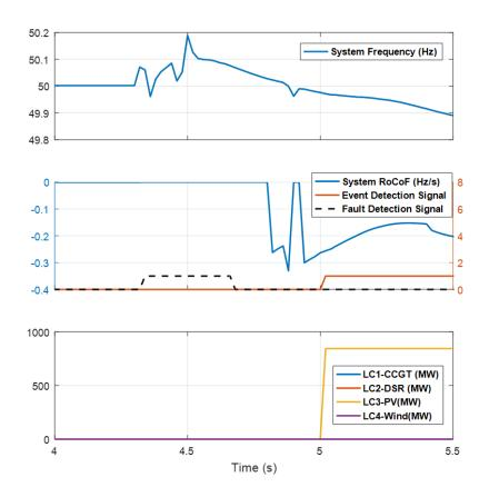
Figure 8-20: Simulation result of generator tripping after a fault at bus 5 of region 1 (zoomed)
