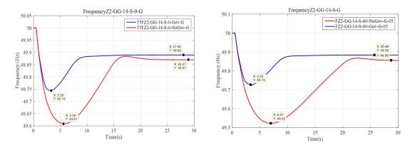
Figure 4-12: Impact of RoCoF relay on frequency response.
