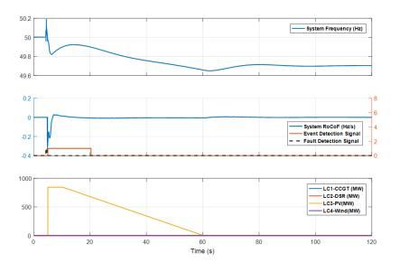
Figure 8-19: Simulation result of generator tripping after a fault at bus 5 of region 1
