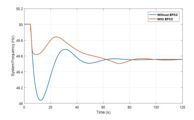
Figure 8-12: System frequency response of a 1500 MW load increase event at bus 9 of region 1.
