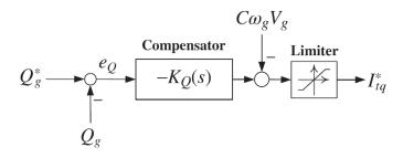
Figure 3-15: A block diagram of reactive power regulator.
