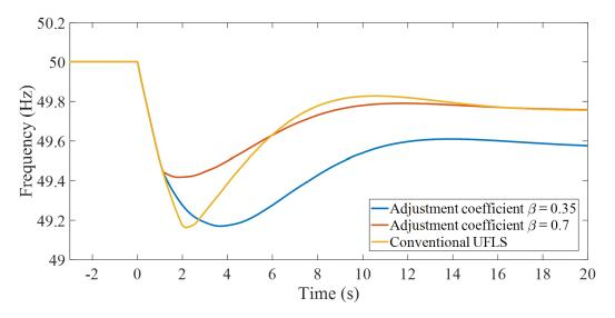
Figure 7-9: The frequency response of the proposed UFLS scheme following LoG events of different size.
