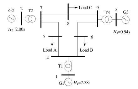
Figure 5-5: Three-machine, 60 Hz test power system.
