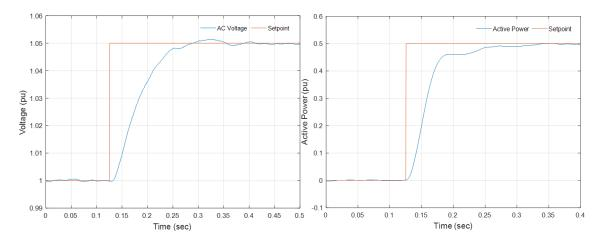
Figure 3-17: Step responses of the AC voltage regulator and active power regulator.
