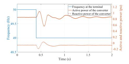
Figure 3-16: Frequency step responses of the converter plant.
