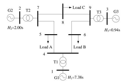
Figure A-2: Single line diagram of IEEE 9-bus test system.
