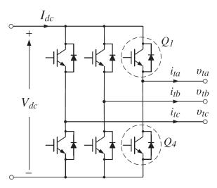
Figure 3-4: Simplified schematic diagram of the two-level VSC
