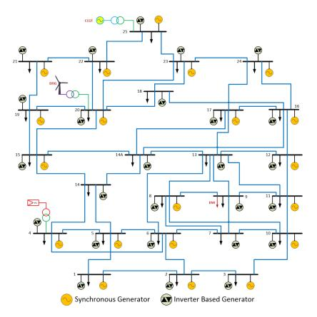
Figure 8-7: Single line diagram of the GB test system.
