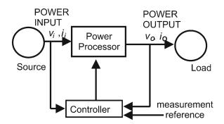
Figure 3-1: A general illustration of power electronics in power system, adapted from [7].
