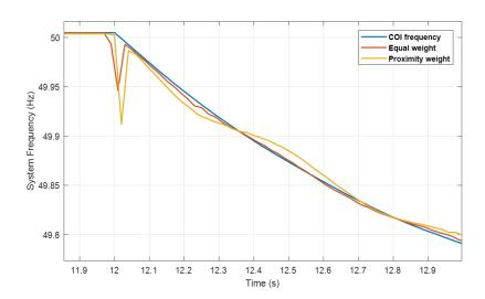
Figure 8-22: System frequency of different PMU weight configurations (zoomed)
