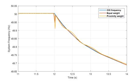
Figure 8-21: System frequency of different PMU weight configurations
