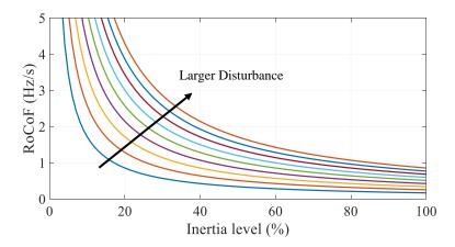
Figure 4-3: Instantaneous absolute RoCoF, a relationship between absolute loss size and inertia.
