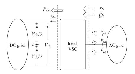
Figure 3-2: A ideal Voltage Source Converter.
