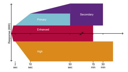
Figure 4-4: Concept for enhanced response service [57].
