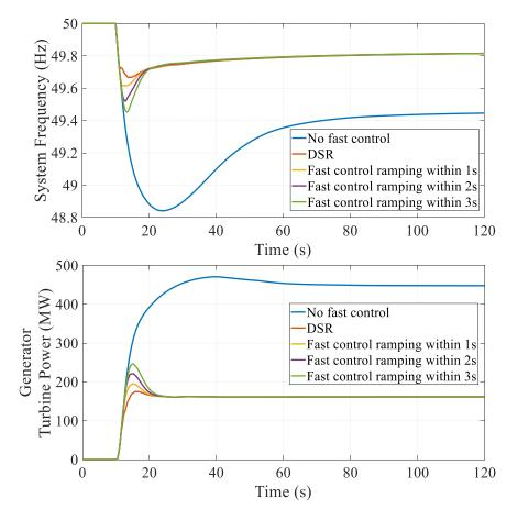
Figure 4-6: Simulation of a 500 MW generation loss in IEEE 39-bus test system with FFR.
