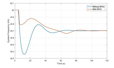
Figure 8-8: System frequency response of a 1000 MW load increase event at bus 9 of region 1.
