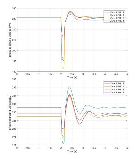
Figure 8-17: Voltages measured by PMU during 140 ms single line ground fault at bus 3 of region 1
