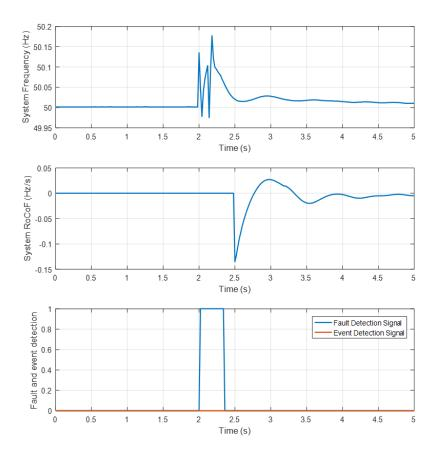
Figure 8-16: Simulation result of a 140 ms single line ground fault at bus 3 of region 1
