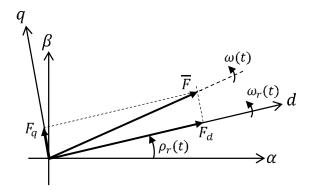
Figure 3-9: Space phasor with the rotating frame.
