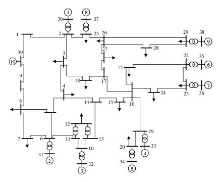
Figure A-3: Single line diagram of IEEE 39-bus test system.
