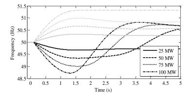
Figure 5-3: Frequencies for a single-machine test system; the black and grey lines denote a load increase and decrease respectively.
