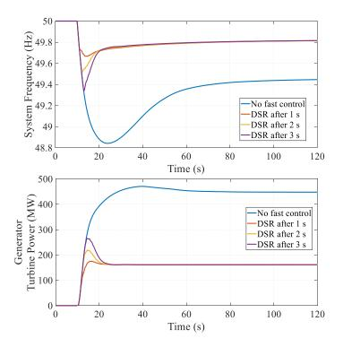
Figure 4-8: Simulation of a 500 MW generation loss in IEEE 39-bus test system with different time delays of FFR.
