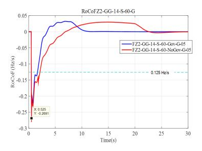
Figure 4-13: Impact of RoCoF relay on system RoCoF.
