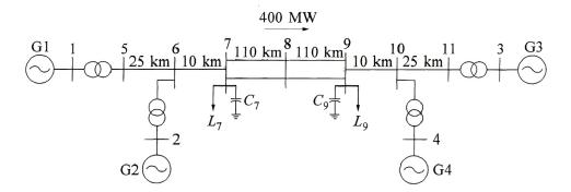
Figure A-1: Single line diagram of Kundur's two area test system.
