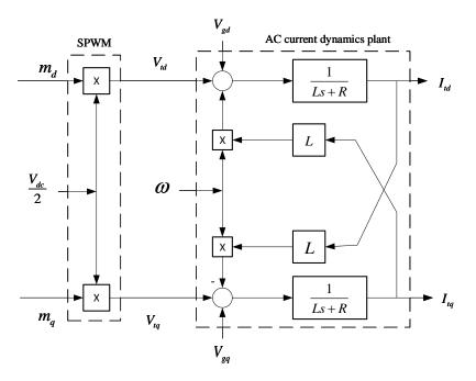
Figure 3-10: The dynamics of the AC side current in dq frame.
