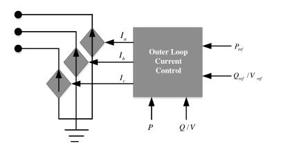
Figure 6-3: PQ power source model in phase reference.
