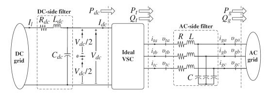
Figure 3-3: Ideal VSC equipped with DC-side and AC-side filters.
