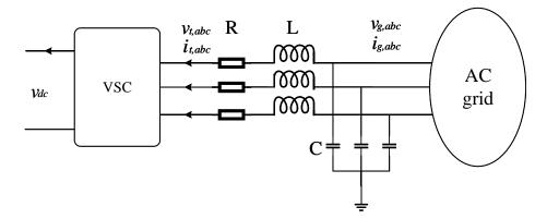
Figure 3-8: Practical VSC converter with filters.
