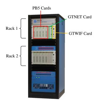
Figure 6-1: RTDS cubic and its key components.
