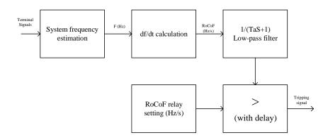
Figure 4-11: Block diagram of the designed RoCoF relay.
