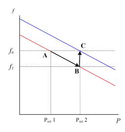
Figure 2-4: Characteristic of primary and secondary control.
