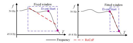
Figure 8-4: Comparison of detection window on RoCoF
