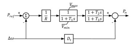
Figure 2-3: A block diagram of a TGOV1 governor controller.
