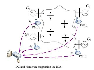
Figure 5-1: A generic WAMS architecture that could support the ICA.
