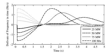
Figure 5-4: Frequency derivatives for a single-machine test system, the black and grey lines denote a load increase and decrease respectively.
