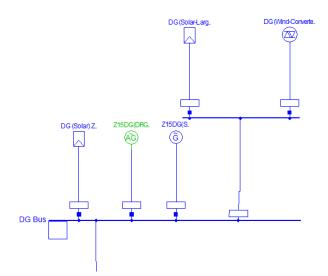
Figure 4-10: Modelling of Distribution Generators in GB 36-zone system.
