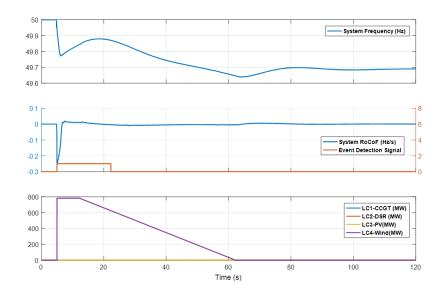
Figure 8-15: Simulation results of a 1000 MW load increase event at bus 21 of region 2
