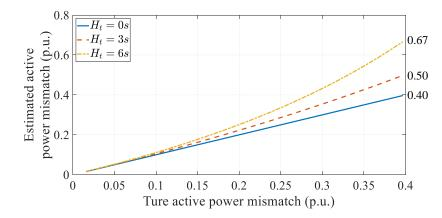
Figure 7-3: Comparison of estimated LoG for different inertia levels of the tripped generator.
