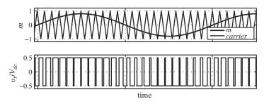
Figure 3-6: The modulating signal, carrier signal, and AC-side terminal voltage, based on the SPWM switching strategy [47].
