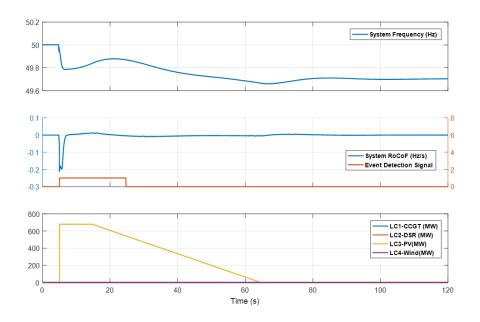
Figure 8-9: Simulation results of a 1000 MW load increase event at bus 9 of region 1.
