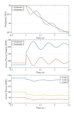
Figure 4-1: Inertia response for loss of 163 MW generation in IEEE 9-bus system.
