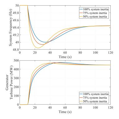
Figure 4-5: Simulation of a 500 MW loss of generation in IEEE 39-bus system.
