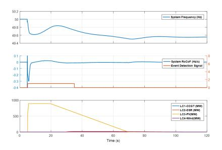
Figure 8-13: Simulation results of a 1500 MW load increase event at bus 9 of region 1.
