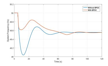
Figure 8-14: System frequency of a 1000 MW load increase event at bus 21 of region 2
