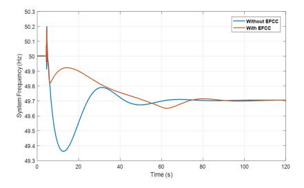
Figure 8-18: System frequency of generator tripping after a fault at bus 5 in region 1
