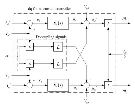
Figure 3-11: A block diagram of the current controller for the system.
