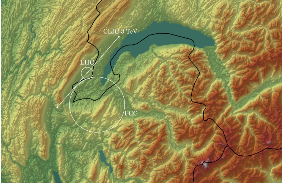
Figure 1.1: The potential locations of CLIC and FCC, with respect to the LHC. The CLIC 3 TeV configuration would be 50 kilometres long. Map produced with Tilemill ( https://tilemill-project.github.io/tilemill/ )
