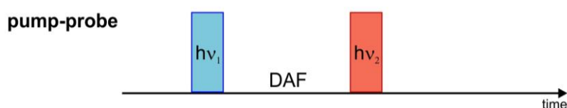
Figure 1.4. Schematic representation of a pump-probe experiment where h\nu_1 is the pump laser pulse (blue) and h\nu_2 is the probe laser pulse (red).
