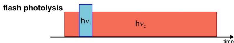
Figure 1.3. Schematic representation of a flash photolysis experiment where h\nu_1 represents the flash responsible for generating the transient species (blue) and h\nu_2 is the probe beam illumination (red).
